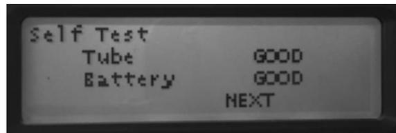
**Step 3:** Reports the overall condition as **GOOD** or **NOT GOOD**, based on the results reviewed in the previous step. Pressing any button will exit the Self-Test and reset the Elapsed Time Clock and dependent subsystems including the Pump Down Data Set—as occurs on any power off state (turned off or batteries dead or missing).
