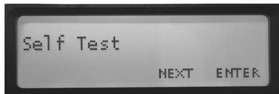
From this Configuration option, press the **ENT** button to enter the “**Self-Test**” sequence. The Self-Test sequence will then start after you press any other button.
