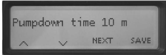
The pumpdown rate is the difference between the start and end of the pressure data shown in the pumpdown graph. For example using a pump down time of ten minutes, a system pump down from atmospheric pressure to one torr in ten minutes has a pump down rate of 760 torr per ten minutes or 76 torr per minute.
