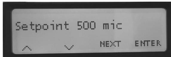
The Set Point indicates a pump down to configured pressure state according to the setting of the Set Point Action. See "Set Point Operation" for more detail.
