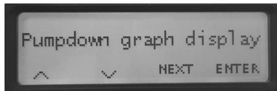
In the example above, the configuration menu is ready to change the display to the Pumpdown Graph. In this state pressing the **ENTER** button will change the display to the Pumpdown Graph, or pressing the **SKIP** button will ignore the state of the menu screen and leave the display mode unchanged.
