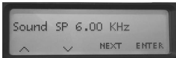
The **Set Point Alarm** sound is typically configured to a different value from the **Calibration Acknowledgement sound**.
