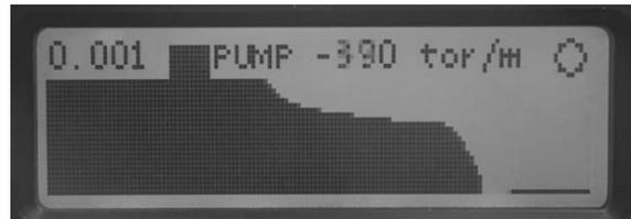
The top left is the **current vacuum pressure** display figure. In the center of the first line is the Vacuum System Analysis, “**PUMP**”, and to the right is one of either the **pump down rate** in units per minute, or the **data set window size** in hours, minutes and seconds. The “**STABLE**” case shows the data set window size.
